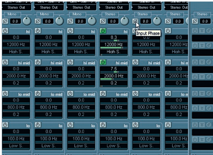
▲ If your tracks are out of phase, you could wind up with reduced frequency content, or even silence. Check the phase in Nuendo with this extremely handy switch
