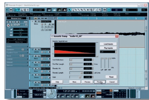
▲ It may not be pretty, and it won't work in real-time, but Nuendo offers a convolution reverb in the form of Acoustic Stamp
